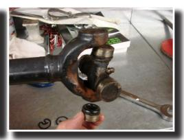
Once the old joint has been removed it is good to clean out the yoke and slightly lube it to assist in installing the new one.
