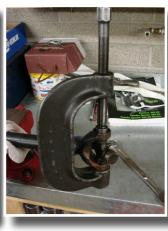
With the clamp we have we just tighten it down and the u-joint gets pressed towards the opposing side of the yoke. If you don't have access to one of these clamps used to press u-joints out you can use a brass drift or a hardened socket (like an impact socket) to drive the old one out. Once the u-joint has slipped out of the yoke you just need to remove one of the needle bearing caps and the u-joint can be removed from the yoke.
